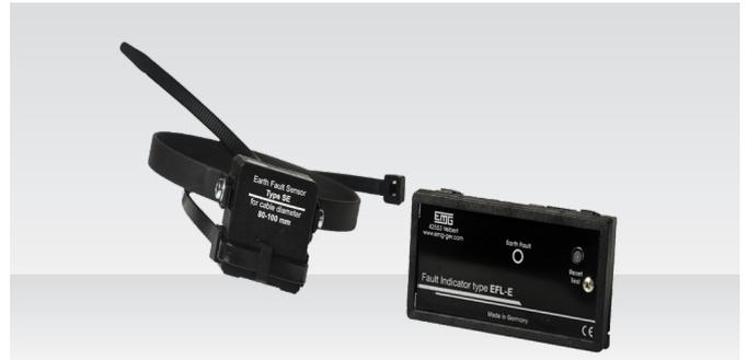
Combined short circuit and earth fault can be also provided. The indicator set consists of one reading instrument, four sensors (one sensor on the 3 core cable and three for the individual 1 core cables) and four fibre optic/standard copper cables. Earth fault and short circuit can be indicated
